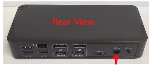
3) Connect your network cable to the docking station. (Does not apply to workstations using Wi-Fi)
